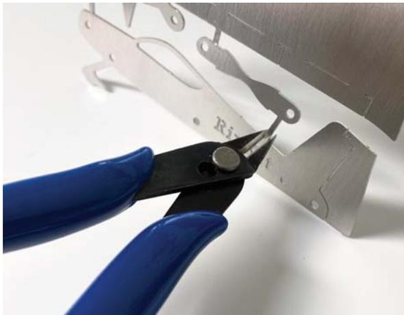
Use a flush cutter to cleanly cut the parts from the factory tree.
