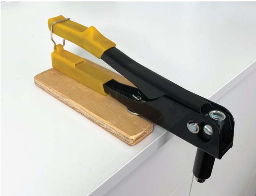
Pushing down on a rivet gun handle is usually easier for smaller hands.
