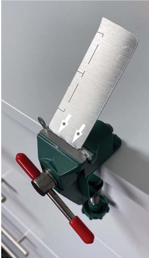
Use a vise or pliers to bend the wings and horizontal stabilizers.
