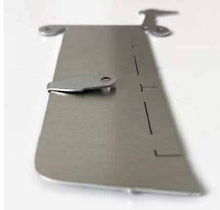
Align the holes of the spinner with a rivet.
